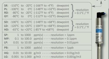
NOTE: ppm, ppb, g/m3 & lbs/MMSCF ranges are stated at atmospheric pressure. Model AMT-Ex Transmitter can be configured to provide corresponding ranges for operation at other constant pressure. This must be stated at time of order.
